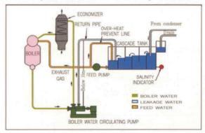
The height of the cascade tank to which the water leaking from the pump is led must be limited to less than 10m in order to reduce pressure on the packing.
